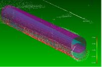
heatmap will not be accurate since it relies upon the As-built geometry as a basis for its calculation. This heatmap only colorizes points from green to red since the relationship to the as-designed surface is corrected and thus we cannot tell "inside" from "outside". This heatmap is best to help visualize the rotation and translation of the as-built location relative to the As-Designed geometry. For large displacements this colorization will effectively be all red.
