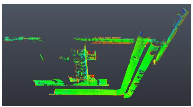
This is a great tool for resolving issues where the as-built models need updating to reflect the field conditions as you're reducing the point cloud down to just the elements that need updating (this file with 27 items is only 9MB) making it simple for CAD/BIM operators to know what to fix.
