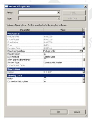
For part parameters, clicking a browse button displays a dialog that makes it easy to map connector parameters to family parameters with the same units. Connector mapping makes the connector parametric with the family.
