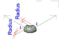
The primary connector of pipe and duct fittings should be located at coordinates (-1, 0, 0). In the following image of the plan view of a P-Trap, connector 1 is the primary connector.
