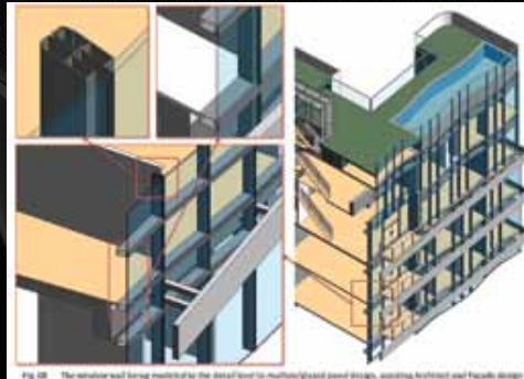
Fig. 08 The window wall being modeled by the detail level to maintain/guard panel design, ensuring Architect and Facade design consistency to ensure the visual impact on site.
