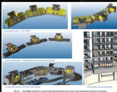
Fig. 22 Revit BIM model for quantity take-off of window wall system, and associated schedule of quantity.
