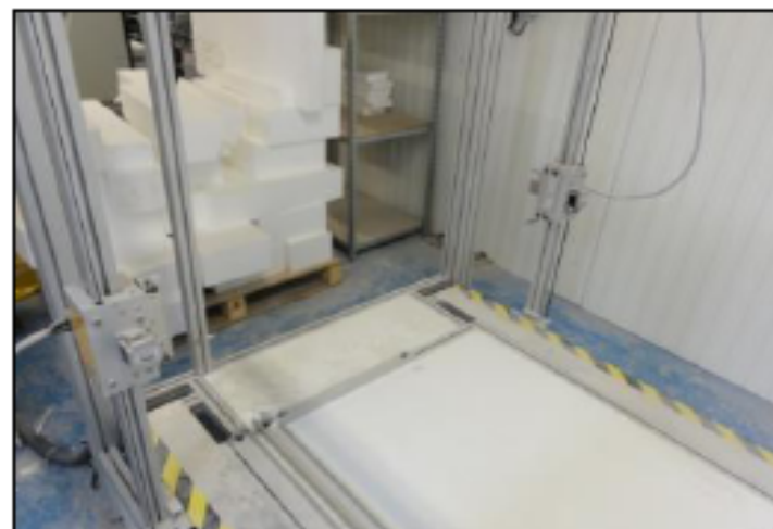
Hot Wire Cutter – for ruled surface panels
