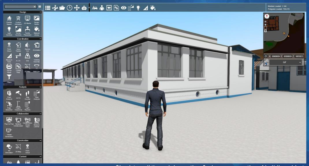
Simulate walkthrough inspection & observe properties of building objects
