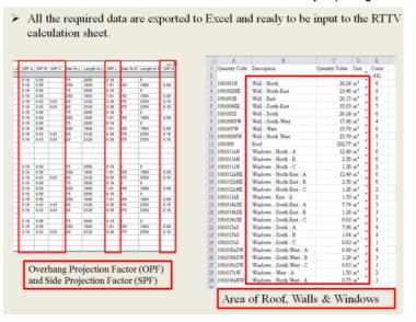
9. The data obtained, including the required external shading coefficients can be exported to the MS Excel to perform detailed calculation.
