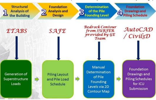
Figure 1 – Workflow of Conventional "One-way" Foundation Design
