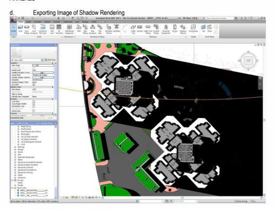
Check and ensure PV panels are not located in shading area
