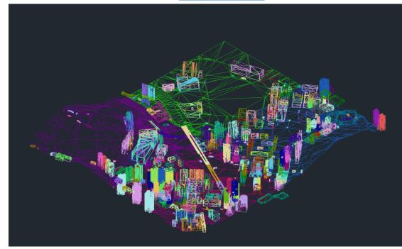
b. In Revit 2016, import the dwg file to fit the site model of Revit file.(Make sure the site model is set to "True North")
