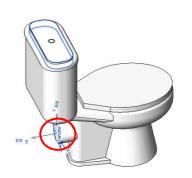
To update the family with new design or adopt the change between design phase and construction phase stated below, load the new family with same family name and insertion point into the project file, the old design will be replaced automatically.
