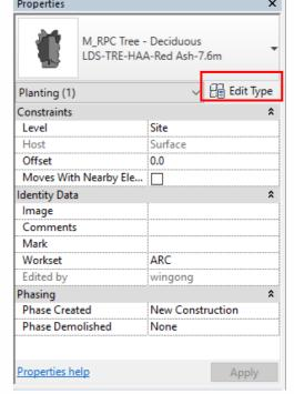
5. In the Type Properties dialog, for Height, enter a value to indicate the new height of the plant and click ok.
