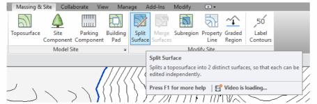
2. Click "Graded Region". In the Edit Graded Region dialog, select Create a new toposurface exactly like the existing one, then select the toposurface. This step demolishes the original surface and creates a copy that occupies the same boundary as the original.
