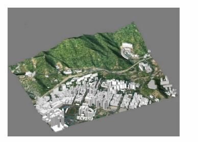
2. Relocate the 3DS model to correct coordinates, and rescale the file to 1:1 (since the files from Lands Department are 1:1000 or 1:5000, normally 1:1000)
