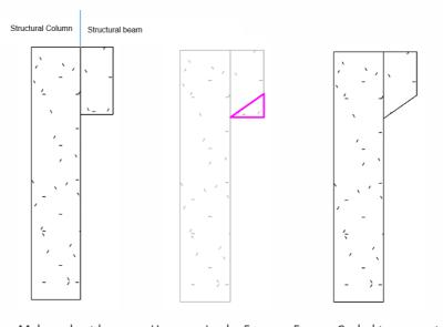
Make a short beam Use opening by Face Form a Corbel to support loading
