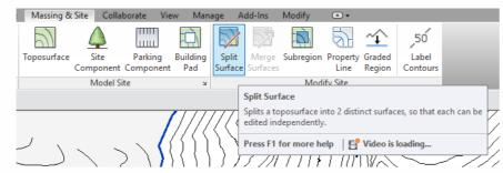
2. Click "Graded Region". In the Edit Graded Region dialog, select Create a new toposurface exactly like the existing one, then select the toposurface. This step demolishes the original surface and creates a copy that occupies the same boundary as the original.
