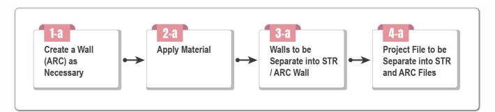
Architects are required to manage 2 models for architectural discipline (ARC models) and structural discipline (STR models) for design and drawing production purposes at early stage;
