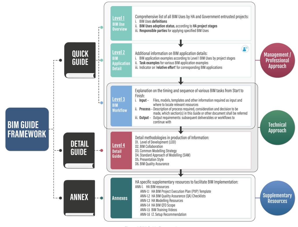
Figure 1 BIM Guide Framework
