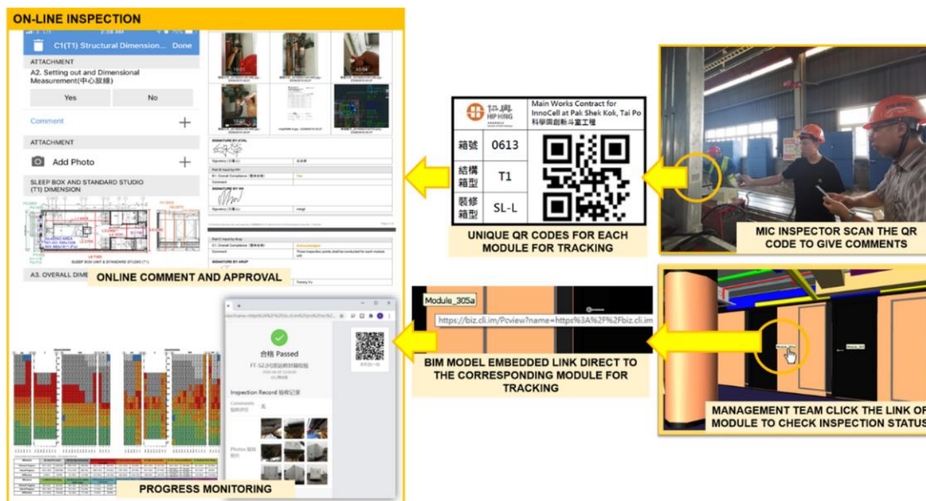
Figure 9.18: Digital platform and e-inspection (Source: Hip Hing Engineering Limited)
