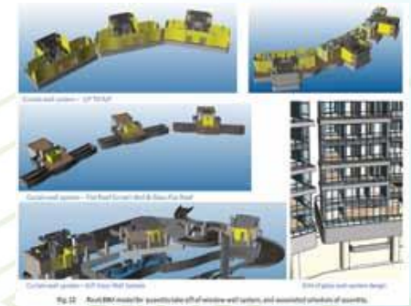
Fig. 10 Revit BIM model for quantifiable QTO of window wall system, and associated schedule of quantity.
