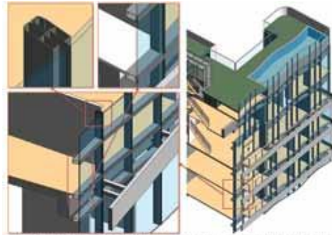
Fig. 08 The window wall being modeled for the detail level for building facade design, including architectural and facade design details for the window wall system.
