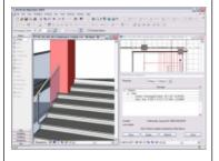
**Interference Check** - Use interference checking to scan your model for collisions between elements
