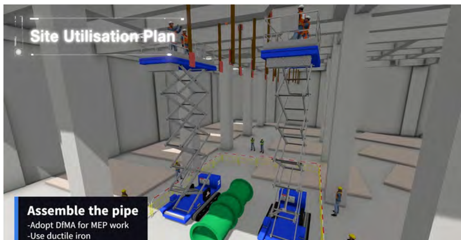
Simulation for Prefabricated pipe module Installation (Developed by Dynamo) Image Courtesy of Paul Y. - Qianhai Joint Venture and Vircon Limited
