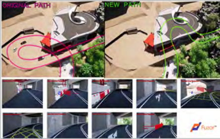
Traffic flow simulation by BIM technology for temporary traffic arrangement coordination with hospital users. Image Courtesy of Architectural Services Department, HKSAR and Shui On Joint Venture and WSP Hong Kong Limited
