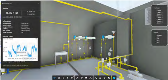
Integration of BIM with IoT for Sensors at Water Treatment Works Image Courtesy of Water Supplies Department, HKSAR Government and Ming Hing Waterworks Engineering Company Limited and Shenzhen Yuegang Technology Company Limited BIM Integration of 2D and 3D within AMIS and 3D Underground Utilities Image Courtesy of Water Supplies Department, HKSAR Government and Ming Hing Waterworks Engineering Company Limited and Shenzhen Yuegang Technology Company Limited
