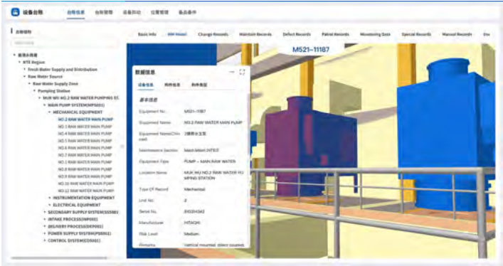
Adoption of BIM in AMIS for Asset Management Image Courtesy of Water Supplies Department, HKSAR Government and Ming Hing Waterworks Engineering Company Limited and Shenzhen Yuegang Technology Company Limited Exploded View of BIM Model in AMIS Image Courtesy of Water Supplies Department, HKSAR Government and Ming Hing Waterworks Engineering Company Limited and Shenzhen Yuegang Technology Company Limited
