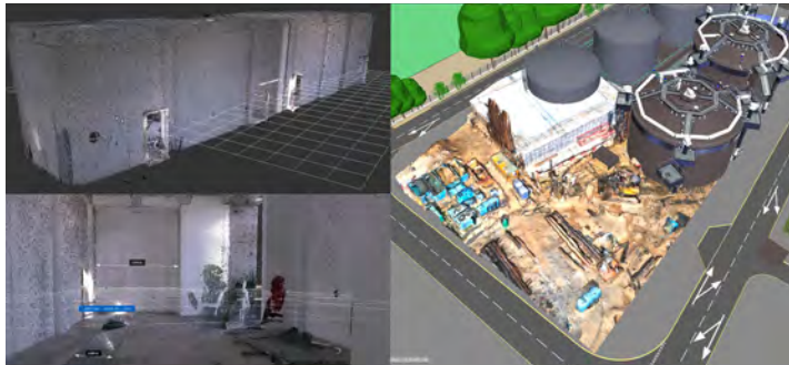
Existing Conditions Modelling using Point Cloud & 3D Photogrammetry Image Courtesy of Drainage Services Department, HKSAR Government and AECOM Asia Company Limited and Paul Y. - CREC Joint Venture and The Jardine Engineering Corporation, Limited
