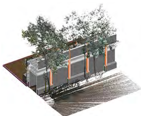
Isometric view of point cloud model of existing trees and BIM model of temporary hoarding. Image Courtesy of Architectural Services Department, HKSAR and Shui On Joint Venture
