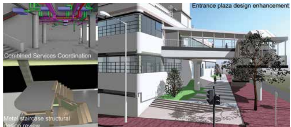
Design and Build BIM Model: The Main Contractor took over the tender model for further updating, enhancement and 3D design coordination. Image Courtesy of Urban Renewal Authority
