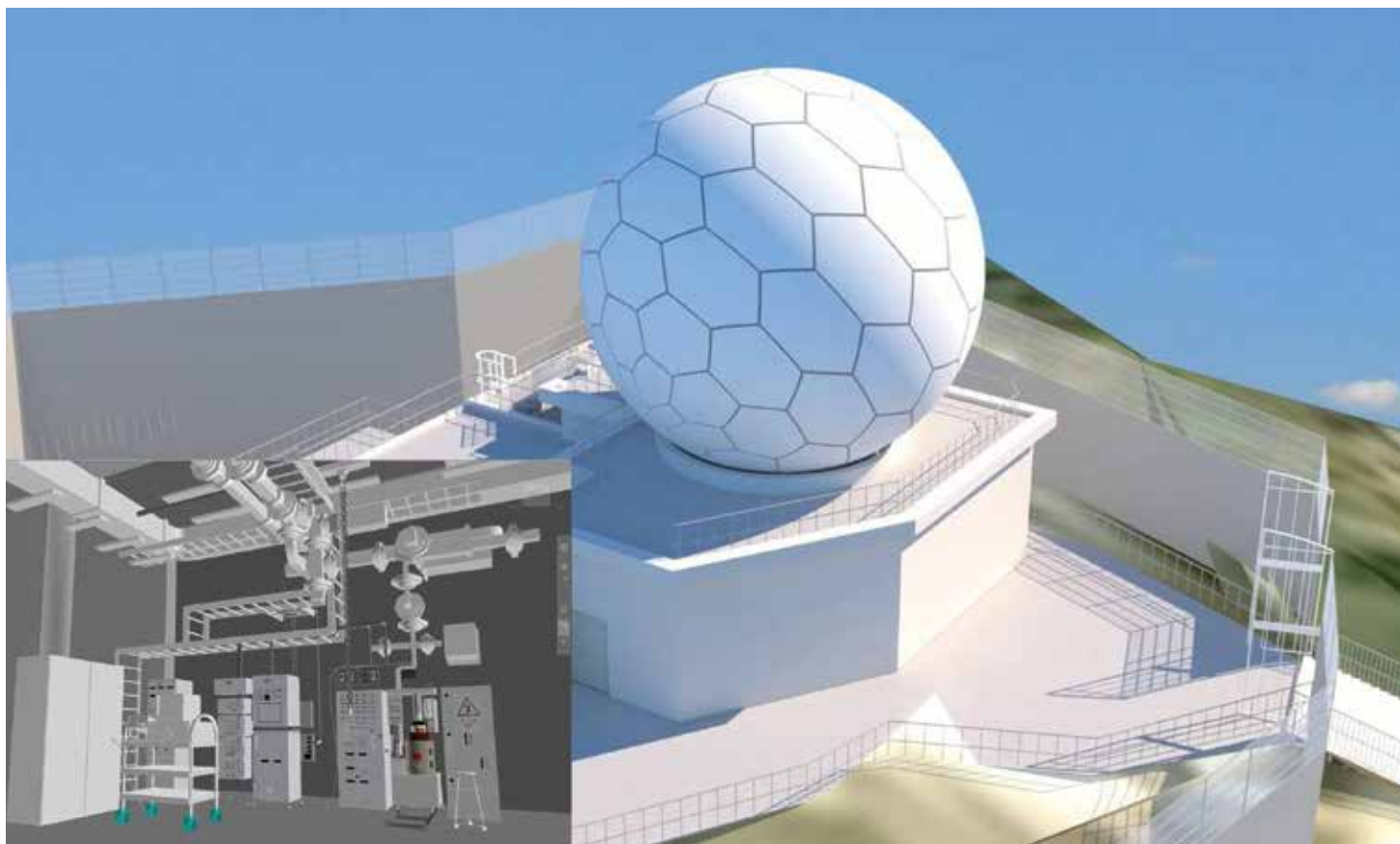
The BIM model of TCWRS. Figure inset shows the equipment room setting inside TCWRS. Image Courtesy of Hong Kong Observatory, HKSAR Government
