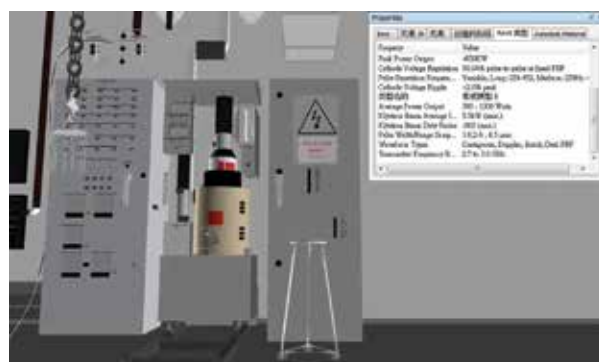
Performance specifications of critical radar equipment embedded in the BIM model. Image Courtesy of Hong Kong Observatory, HKSAR Government
