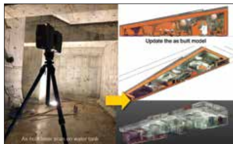
As-built BIM Model updated based on as-built laser scan data for proper documentation. Image Courtesy of Urban Renewal Authority
