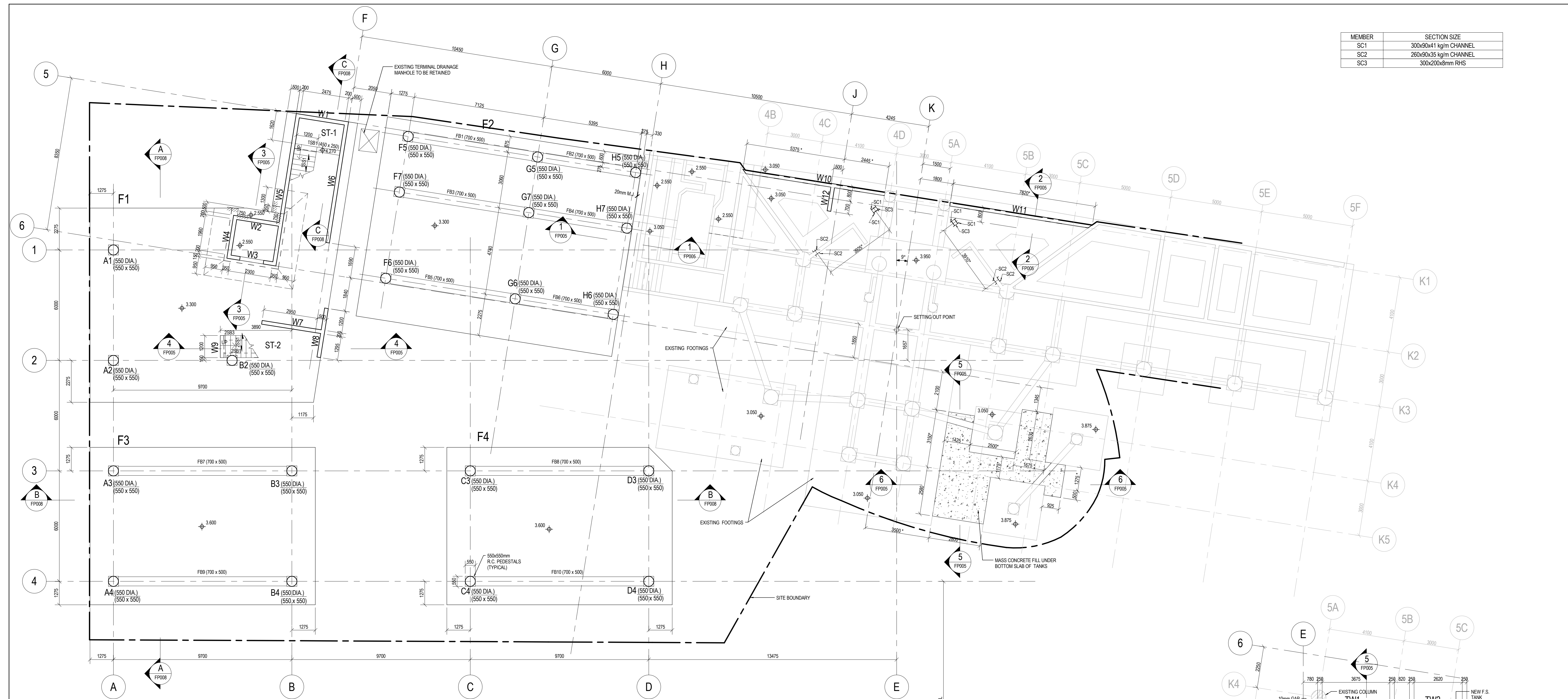
FOUNDATION PLAN (1 : 100) UNLESS OTHERWISE STATED: 1. ALL NEW FOOTINGS TO BE 350mm THICK. 2. ALL NEW R.C. WALLS TO BE 200mm THICK. 3. \phi DENOTES THE TOP LEVEL OF THE FOOTINGS.
