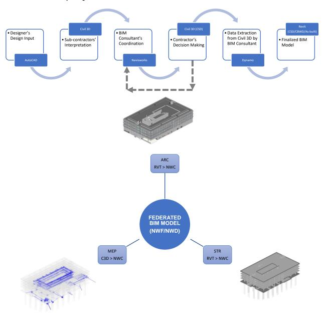
BIM manager will then create a Federated BIM Model by combining ARC, STR and MEP BIM Models, and conduct the clash detection analysis. Clash detection are run with Autodesk Navisworks Manage.
