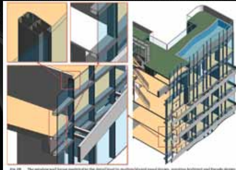
Fig. 08 The window wall being modeled by the detail level to maintain/guard panel design, existing Architect and Facade design consultant to ensure the visual impact on site.
