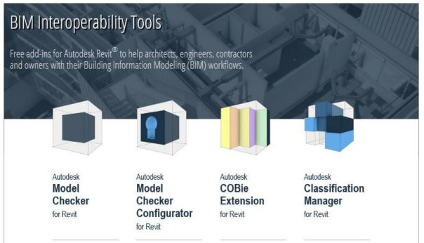
Revit includes free add-in toolkits to validate that the model is COBie compliant, and to extract COBie data from the model
