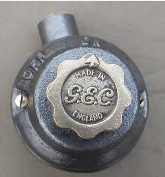
Similar single pole rotary switch manufactured by the General Electric Company in the 1930s in England. (Unknown, Auctiva Emporium: SPIDYLODGE20 2015)
