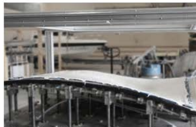
3.1 – Casting verified panel
