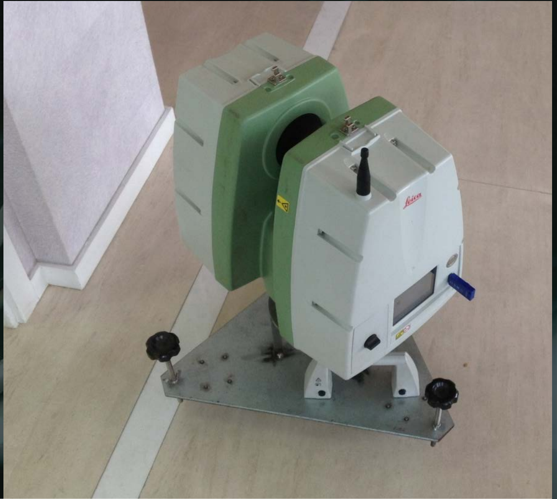
Laser Scanner - 50,000 pts /s; Range: 300m; Accuracy 6mm
