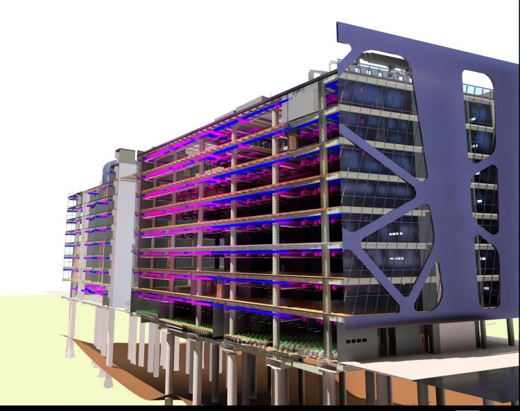
Sectional perspective of federated BIM model
